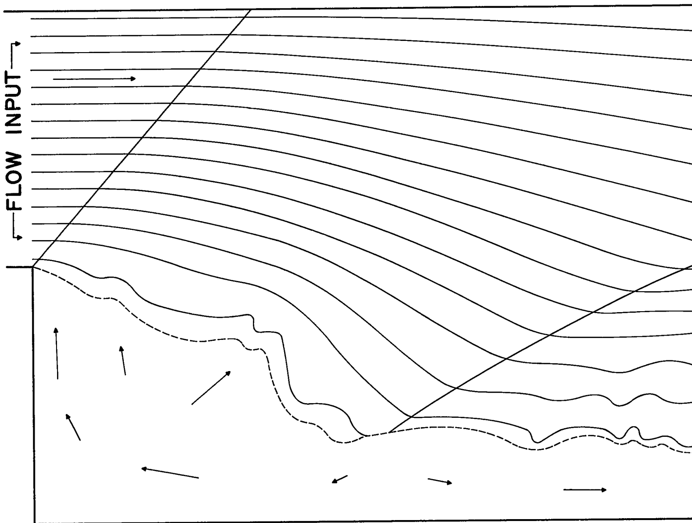
Fig. III-9 Configuration of the flow pattern at t = 70 for the calculation for helium, showing mass-point lines, region of turbulence with shock reflected therefrom, Mach line from corner, and some local-velocity vectors.
